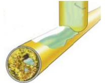
**Garbage disposals** don't keep grease out of your pipes—they chop the food into small pieces, leaving the grease. **Drain cleaners** dissolve grease in your drain but send the grease further down where a new clog can develop.
